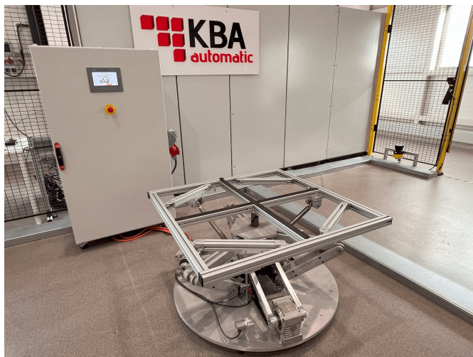
Fig. 4. The real-life Stewart-lift platform [source: authors]
