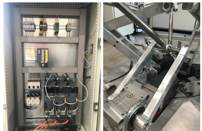
Fig. 6. Control and executive elements of the platform [36]
