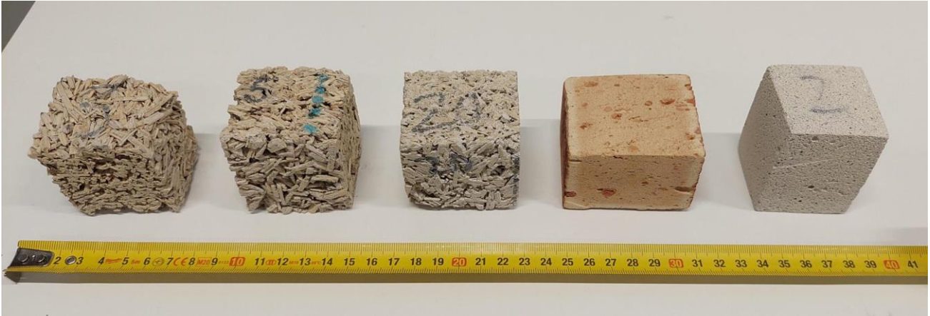
Fig. 2. Archimedes test samples (from the left: D300, D500, PCM20, red brick, and autoclaved aerated concrete).
