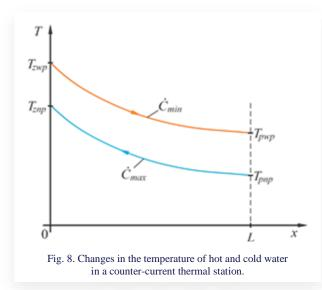
Heat flow rate  $\dot{Q}_m$  in formula (4) was calculated as the arithmetic mean of heat flux  $\dot{Q}_{wp}$  given off by hot water and heat flux  $\dot{Q}_{np}$  absorbed by cold water. The following formula was used to calculate the heat flow rate transferred from the water with a higher temperature (water from the heat distribution network):
