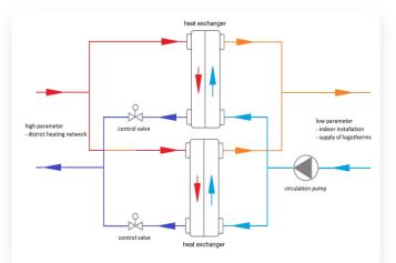
Fig. 7. Schematic diagram of the thermal node from which the data was obtained.
