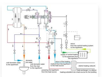
Fig. 1. Diagram of a logotherm fed from a heat exchanger in a district heating substation [11].
