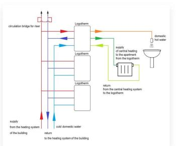
Fig. 4. Diagram of the clip installed at the end of the heating riser.
