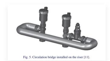
The clips mounted within logotherms operate based on the same principle as the circulation bridges mounted on the internal system risers. This enables the flow of the heating medium close to the logotherm, thus shortening the time of waiting for the heat needed to supply the substation. If the heating medium cools down in the branch feeding the substation, the valve opens, forcing the heating medium flow to the branch returning to the source of supply.
