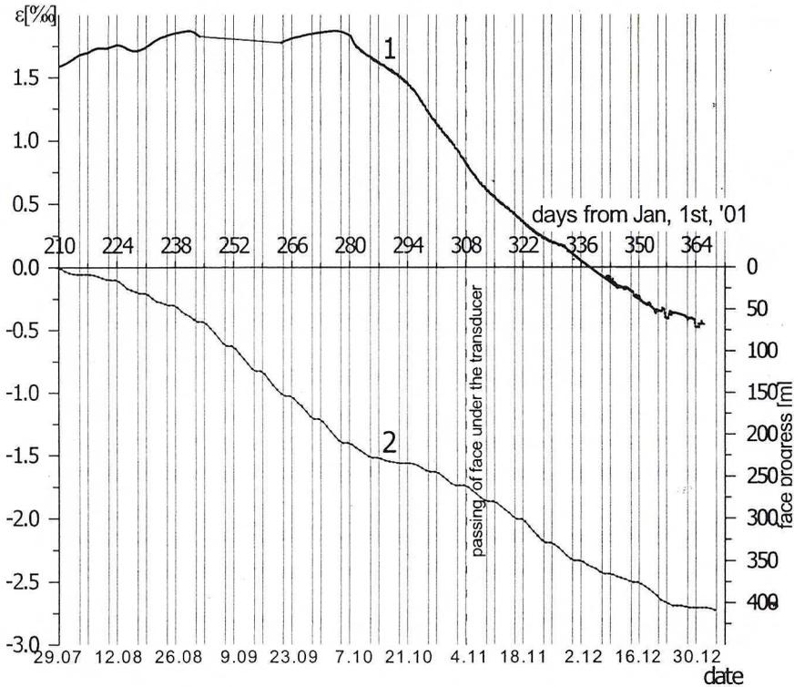
Fig. 15. The "Ziemowit" coal mine. Horizontal strains measured by transducer 8 (1) and face progress (2)
