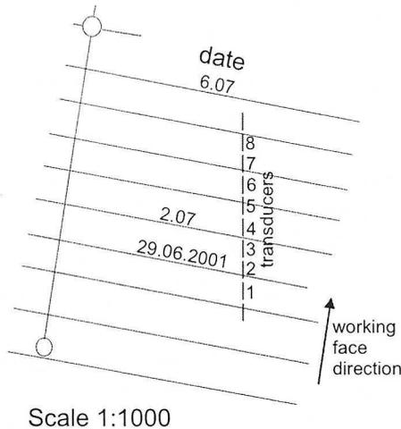
Fig. 3. The layout of strain transducers (“Wesoła” coal mine)
