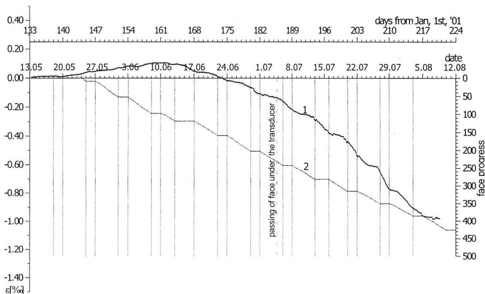
Fig. 13. The “Wesoła” coal mine. Horizontal strains measured by transducer 8(1) and face advance (2)
