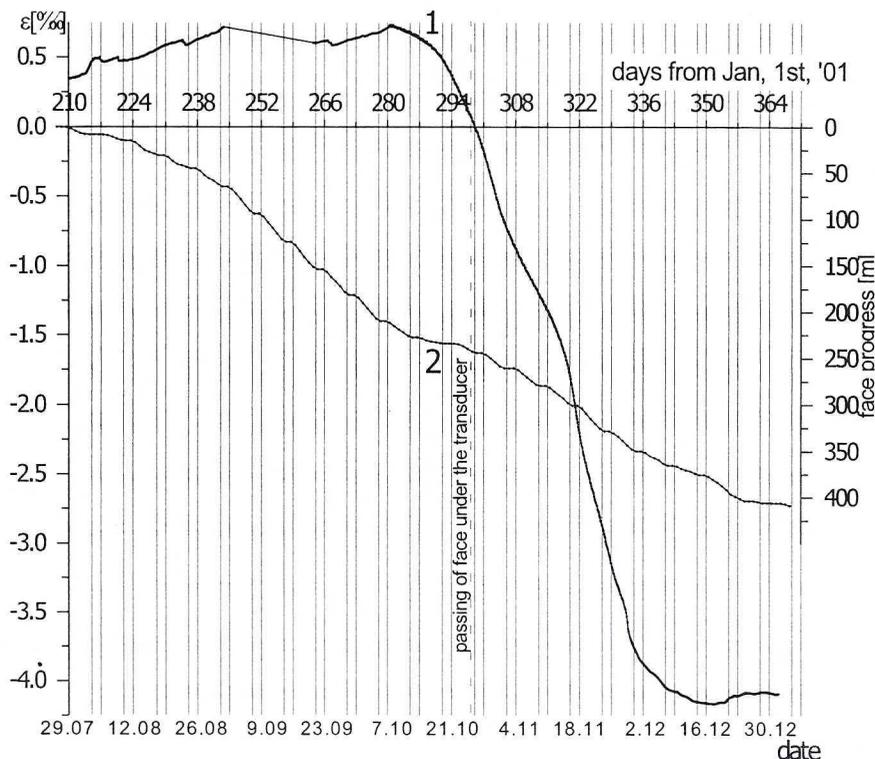
Fig. 14. The "Ziemowit" coal mine. Horizontal strains measured by transducer 6(1) and face progress (2)
