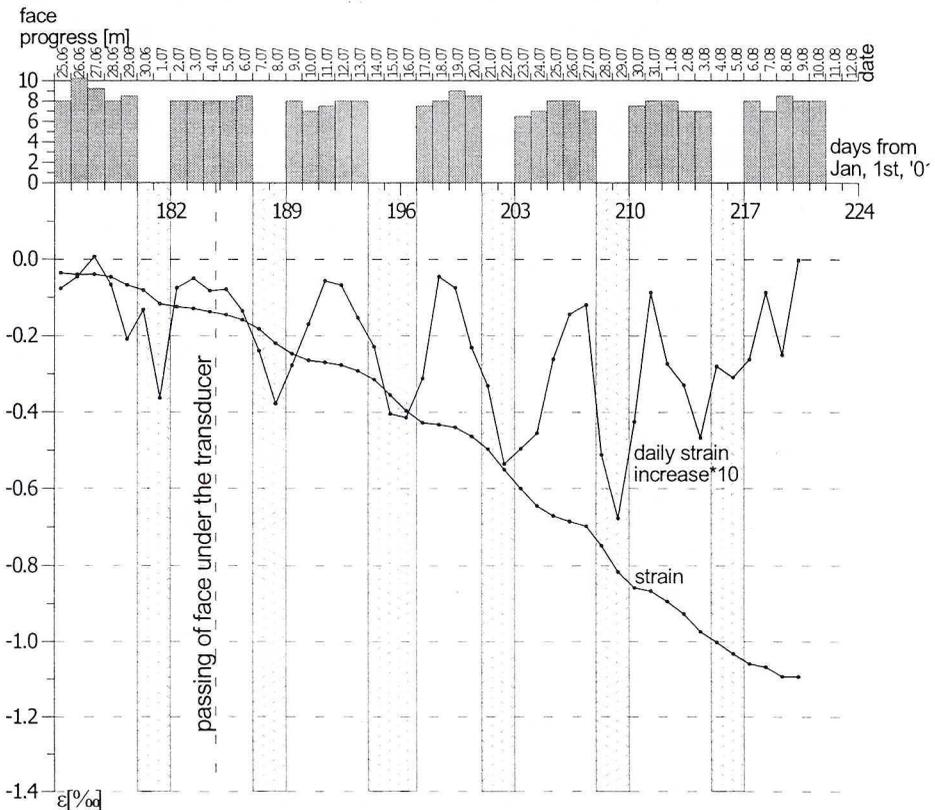
Fig. 7. The “Wesoła” coal mine, transducer no. 7. The strain and its daily increase with measurements taken every 24 hours
