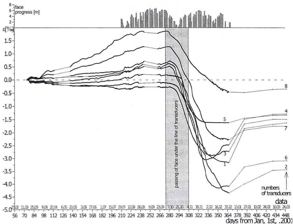
Fig. 9. The “Ziemowit” coal mine. Soil strain as a function of time
