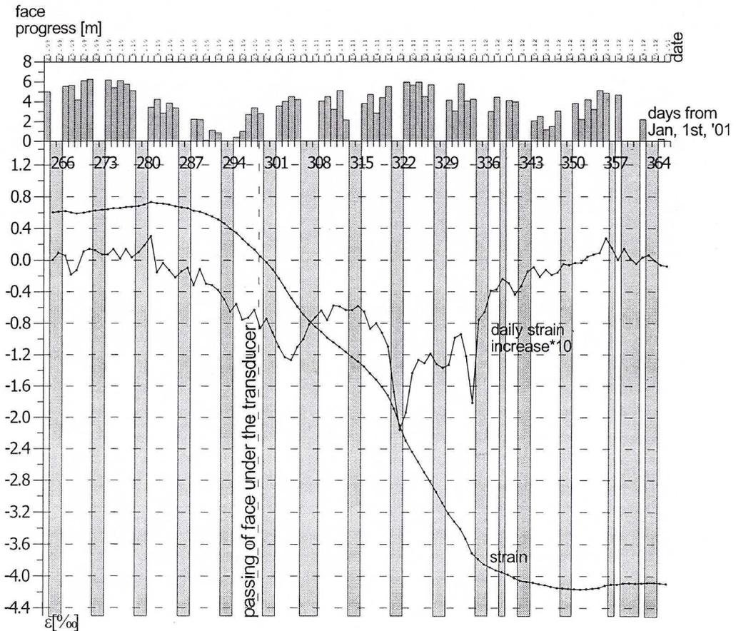
Fig. 10. The “Ziemowit” coal mine, transducer no. 6. The strain and its daily increase with measurements taken every 24 hours
