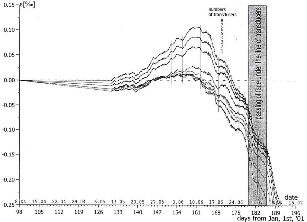
Fig. 16. The “Wesoła” coal mine. Strains as a function of time, measured till July 15<sup>th</sup> 2001
