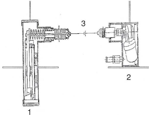
Fig. 1. Transducer to measure displacements and temperature; type TTCS-4000.3
