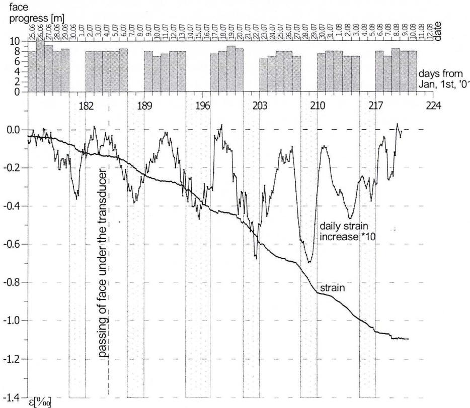
Fig. 8. "Wesoła" coal mine, transducer no. 7. The strain and its daily increase with measurements taken every 3 hours
