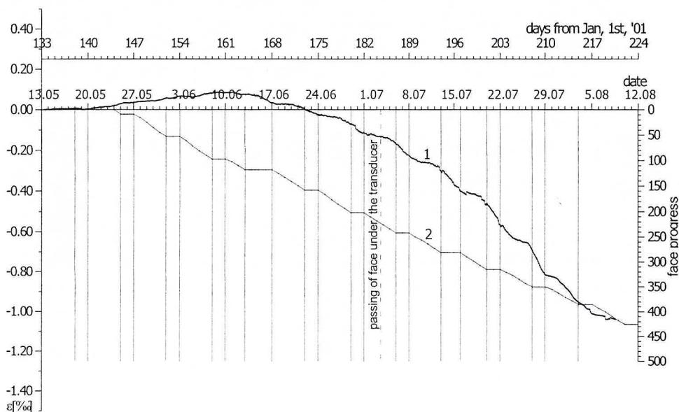
Fig. 12. The “Wesoła” coal mine. Horizontal strains measured by transducer 6(1) and face advance (2)
