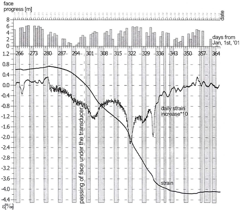
Fig. 11. The “Ziemowit” coal mine, transducer no. 6. The strain and its daily increase with measurements taken every 3 hours
