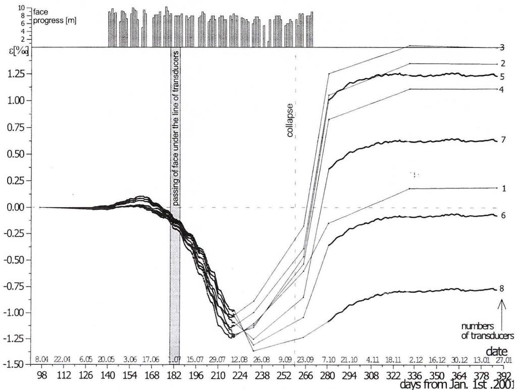
Fig. 6. The “Wesoła” coal mine. Soil strains as a function of time
