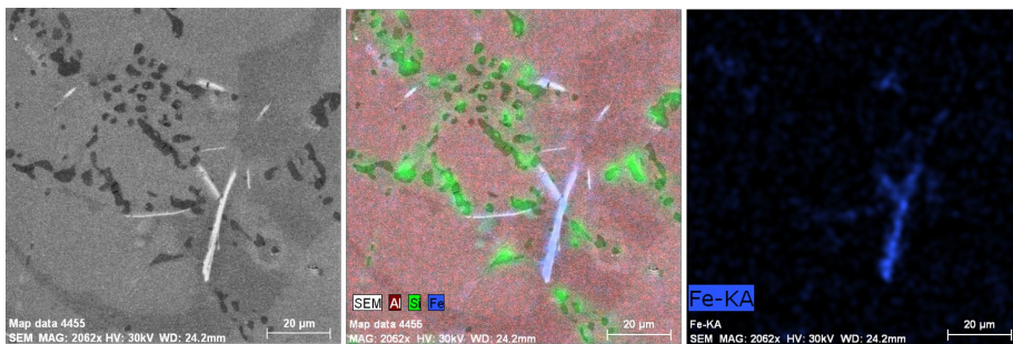
Fig. 11. Fe-rich intermetallic phases with corresponding EDX mapping of chemical elements (Ti-0.3, T6, H 2 SO 4 etch.), SEM
