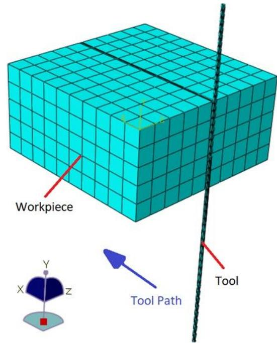
Fig. 2. The workpiece's and tool's undeformed model meshing
