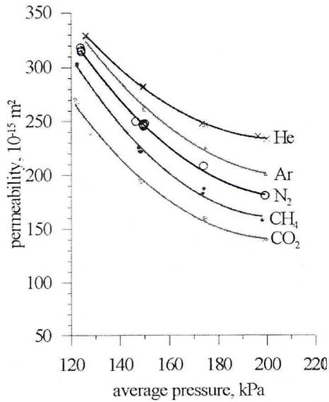
Fig. 8. The permeability variations in sample W02 with the increase of gas pressure
