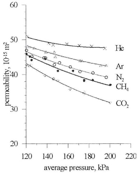
Fig. 7. The permeability variations in sample W01 with the increase of gas pressure
