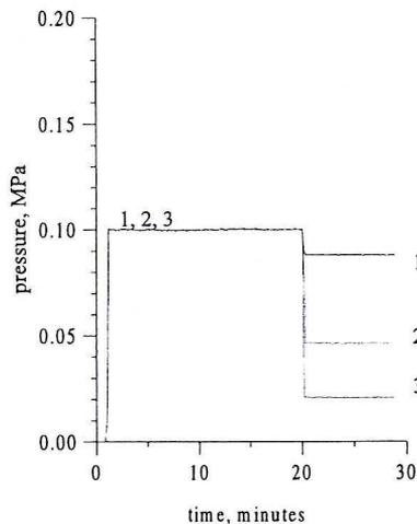
Fig. 3. The pressure variations in sample W01 during its saturation with helium and its flow
