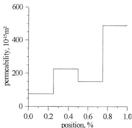
Fig. 5. The variations of permeability in different parts of the sample W02
