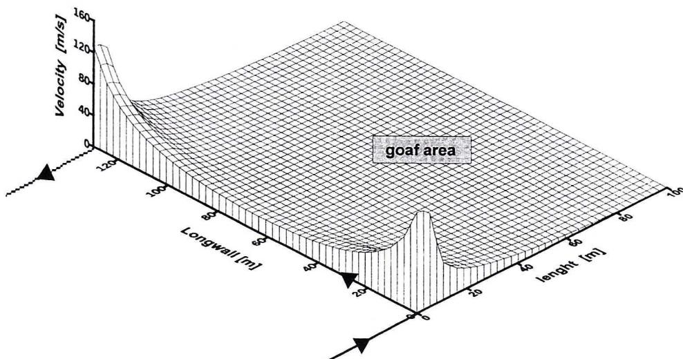
Fig. 4. Distribution of the modulus of flow velocity in goaf — example A — computer simulation
