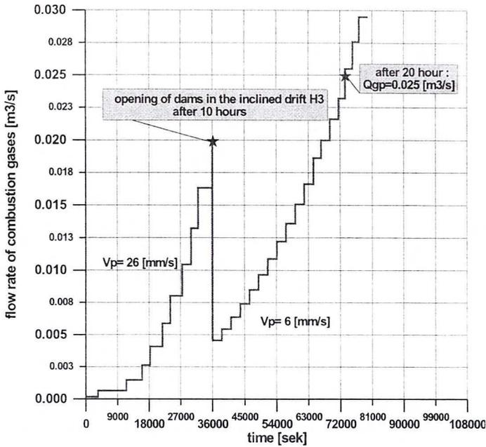
Fig. 10. Flow rate of combustion gases generated in the fire
