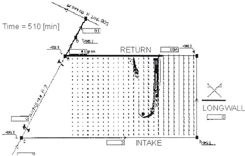
Fig. 8. Spatial diagram of the network of excavations — computer simulation, fire in goaf (isopleths of combustion gases concentration levels, lines of stream for the flow in goaf)
