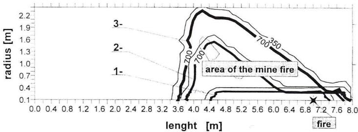
temperature isopleths of the mine fire - Tog thick line = 700 [K],
