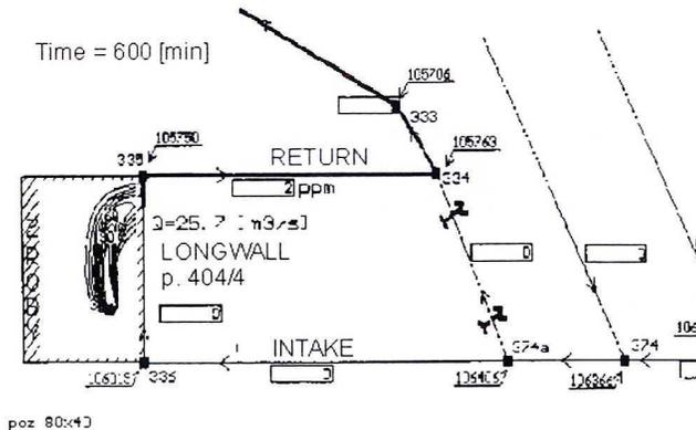
Fig. 2. Spatial diagram of the network of excavations — computer simulation — fire in goaf, isopleths of concentration levels of combustion gases
