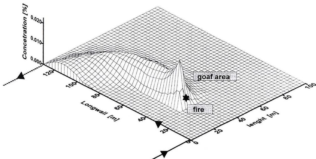
Fig. 3. Distribution of concentration levels of combustion gases in goaf — computer simulation
