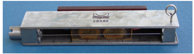
Fig. 2. A VW strain gauge with the ends of the wire directly anchored to the tested object
