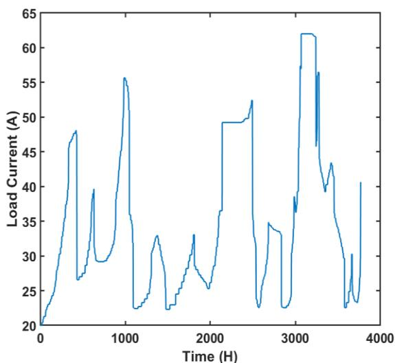
**Fig. 11** Load current profile for variable load condition test
