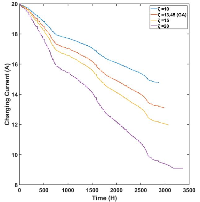
Fig. 8 Charging currents under different weighting parameters for constant load condition test
