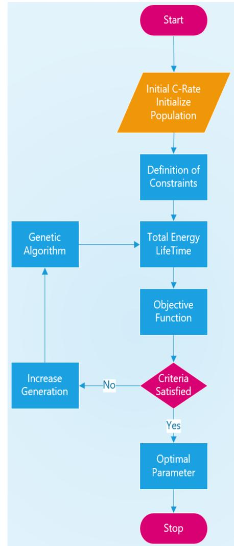
Fig. 5 Genetic Algorithm Optimization Flowchart
