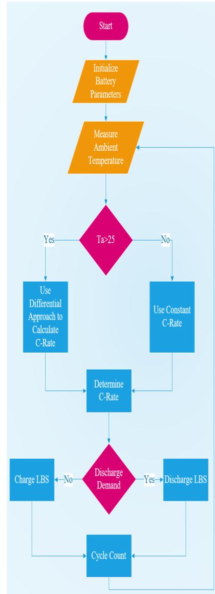
Fig. 1 Flowchart of the proposed battery management approach
