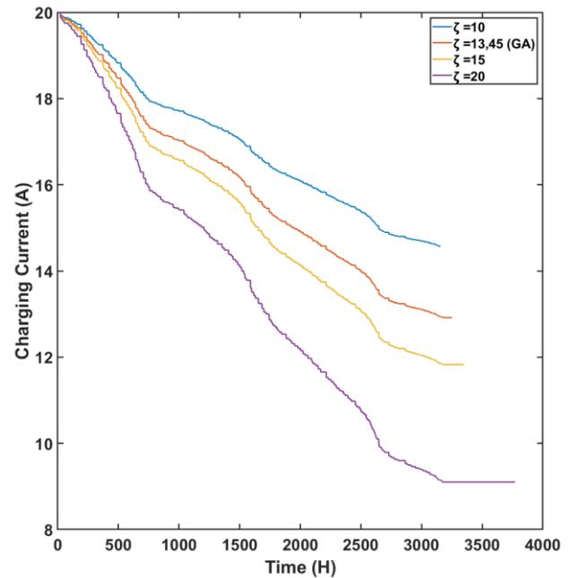
**Fig. 12** Charging currents under different weighting parameters for variable load condition test
