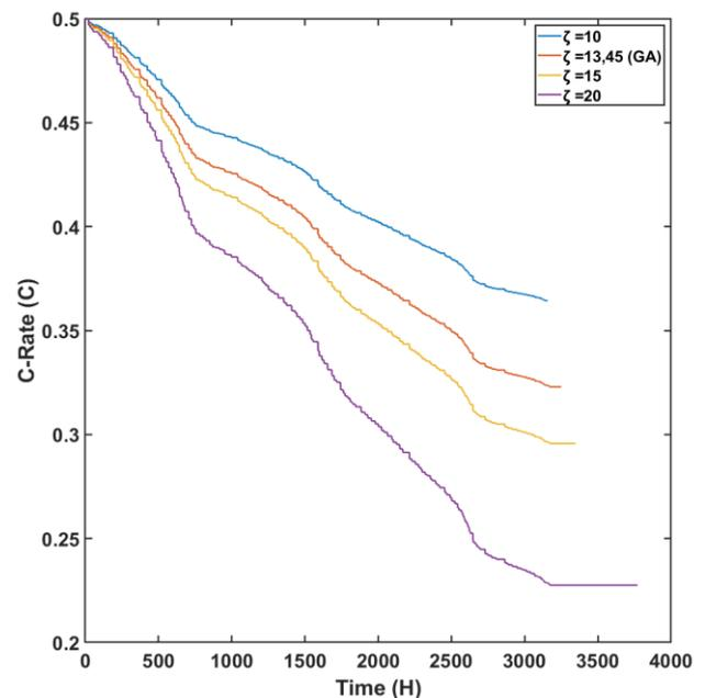
**Fig. 13** C-Rate values under different weighting parameters for constant load condition test
