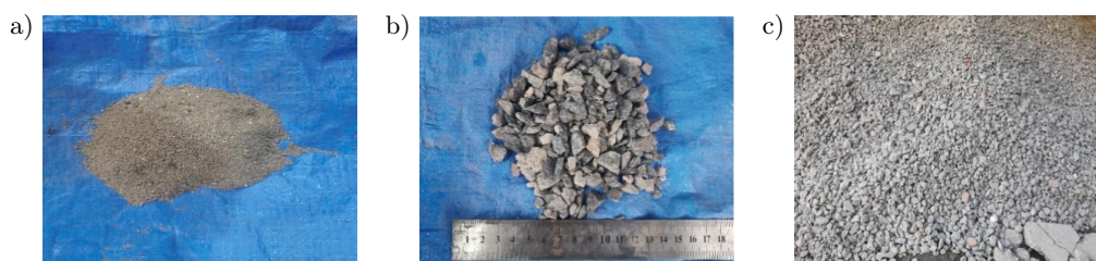
Fig. 1. Coarse and fine aggregates of RAC: a) fine aggregates; b) natural coarse aggregates; c) recycled coarse aggregates.
