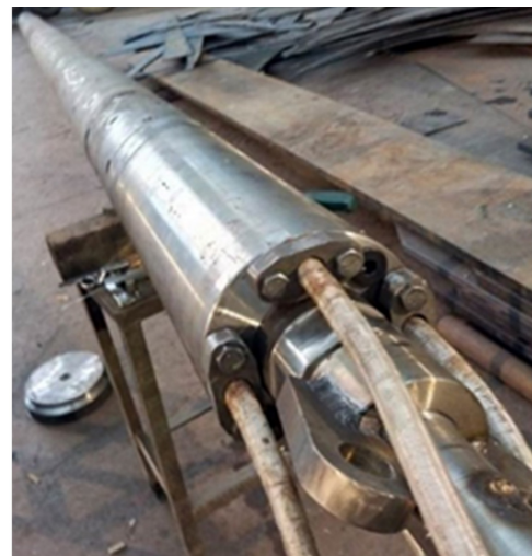
Fig. 15. The electric heater prototype completed
