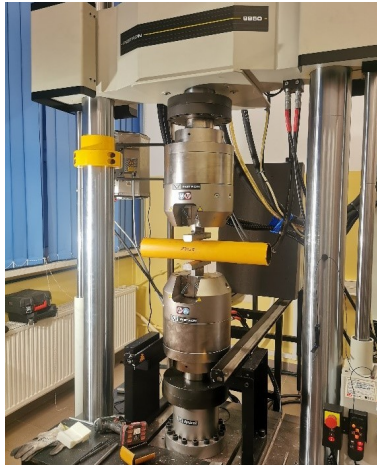
Fig. 22. Instron 8850 machine with tested sample
