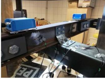
Fig.8. The inclinometers location on the tested specimen
