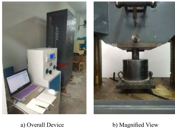
Fig. 9. Experimental setup for quasi-static loading test of a wolframite ore
