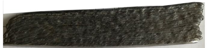
Fig. 7. Specimen obtained by WAAM
