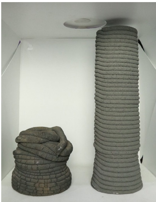
Fig. 16. Printing test results of W14 (left) and W14F (Right)
