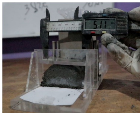
(c) Measuring width using Vernier scale
