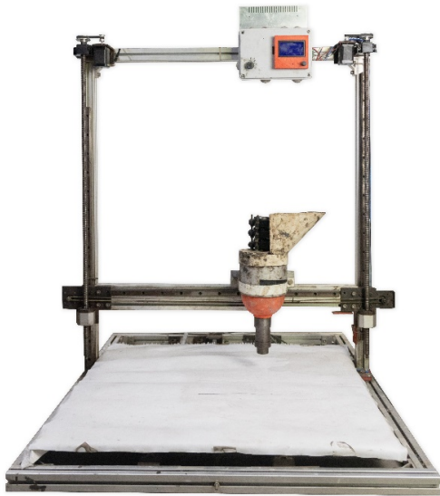
Fig. 3. A 1×1×1 m 3D concrete printer
