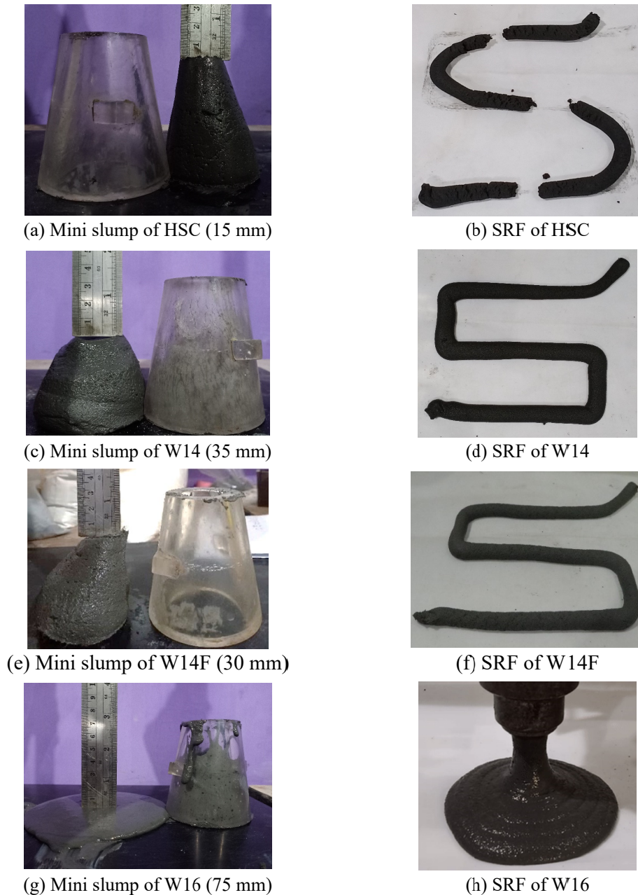
Fig. 10. The connection of mini slump and SRF form of each sample
