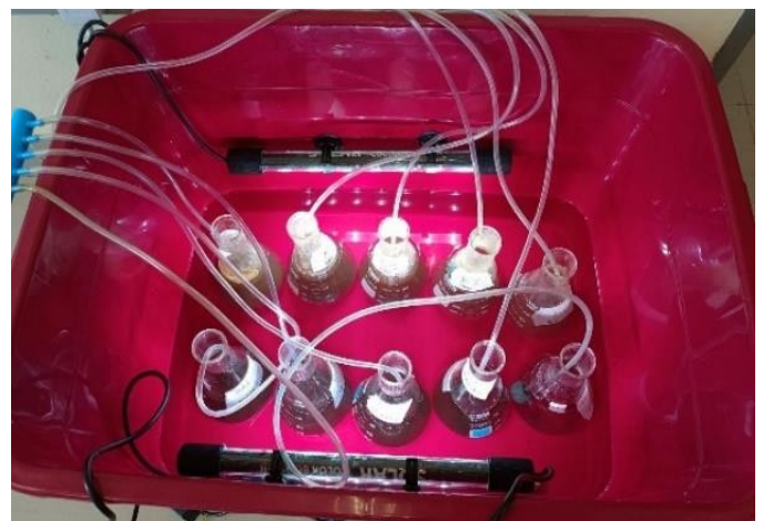
Fig. 4. Full setup for cultivation of microalgae with pumps and oxygen stones
