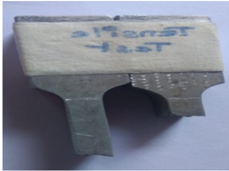
Fig. 2. (a) Tensile test sample of Al6061 HMMC for the load of 40 KN
