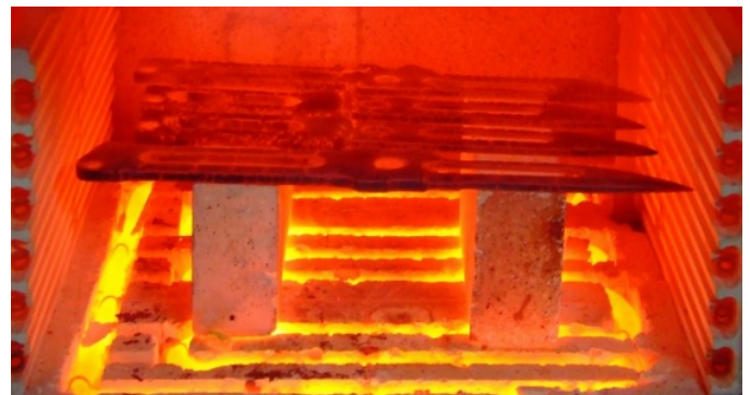
Fig. 3. Heat treatment in a Muffle furnace temp range of 300°C to 1,200°C
