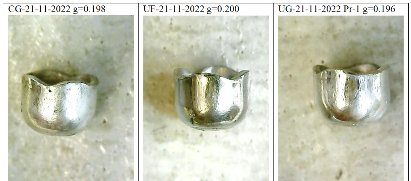
Fig. 10. Obtained micro cups for three series of material with information about the exact thickness g of the foil used
