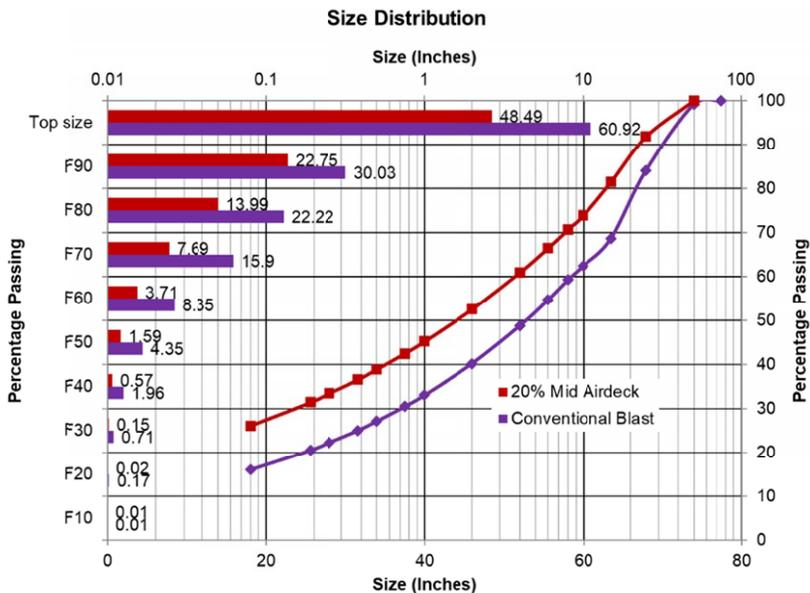
Fig. 13. Comparison of percentage passing of fragmentation of conventional and mid-air deck blast for different sieve sizes at Bench-3
