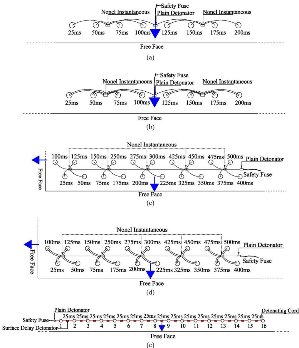
Fig. 4. Firing pattern for Bench-1: a) full-column, top and bottom air deck, b) mid-air deck; Bench-2: c) full-column, d) mid-air deck; and Bench-3: (e) both full-column and mid-air deck positions
