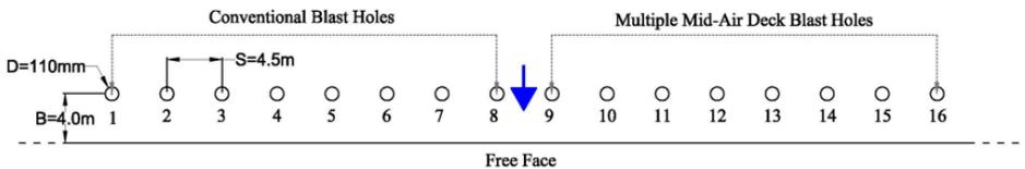
Fig. 5. Drill hole pattern at the experimental Bench-4
