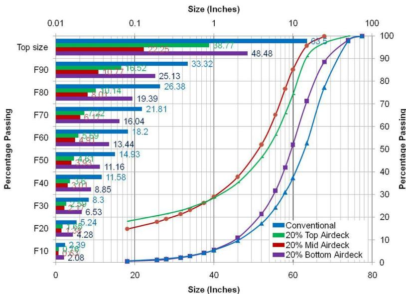
Fig. 9. Comparison of % passing size distributions for conventional and 20% air deck lengths at various positions within the explosive column at Bench-1
