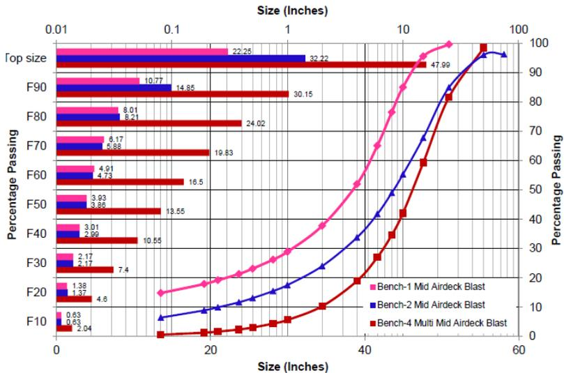
Fig. 16. Comparison of percentage passing of fragmentation of mid-air deck and multiple mid-air deck blasts
