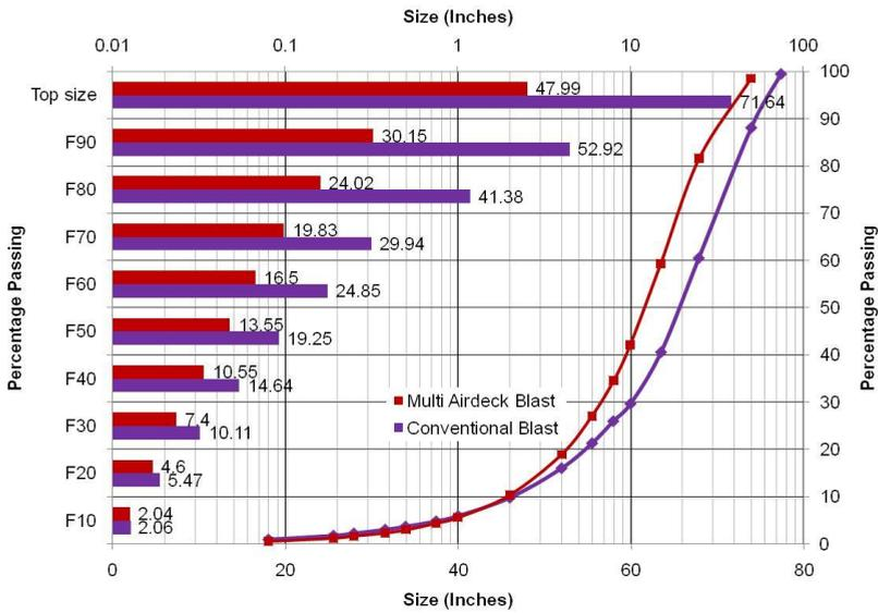
Fig. 15. Comparison of percentage passing of fragmentation of conventional and multiple mid-air deck blast for different sieve sizes at Bench-4
