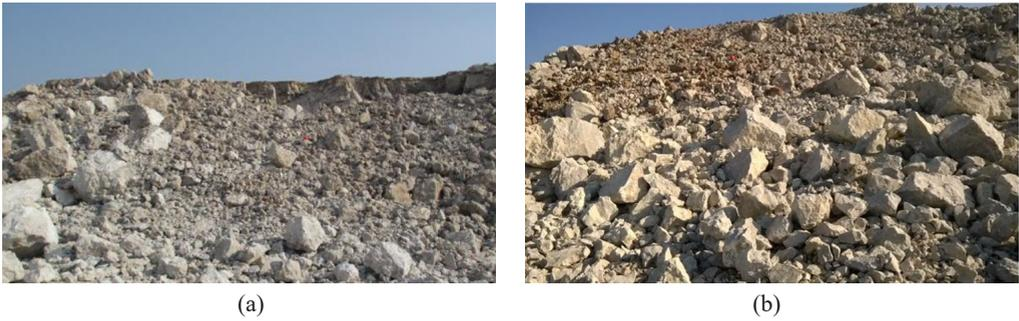
Fig. 10. Comparison of full-column charge blast fragmentation and 20% mid-air decks at Bench-2
