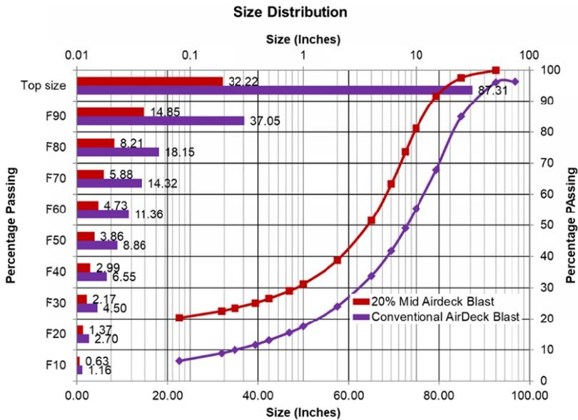
Fig. 11. Comparison of percentage passing of fragmentation of conventional and mid-air deck blast for different sieve sizes at Bench-2
