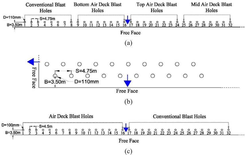
Fig. 1. Drill hole pattern at the (a) Bench-1 (b) Bench-2 and (c) Bench-3
