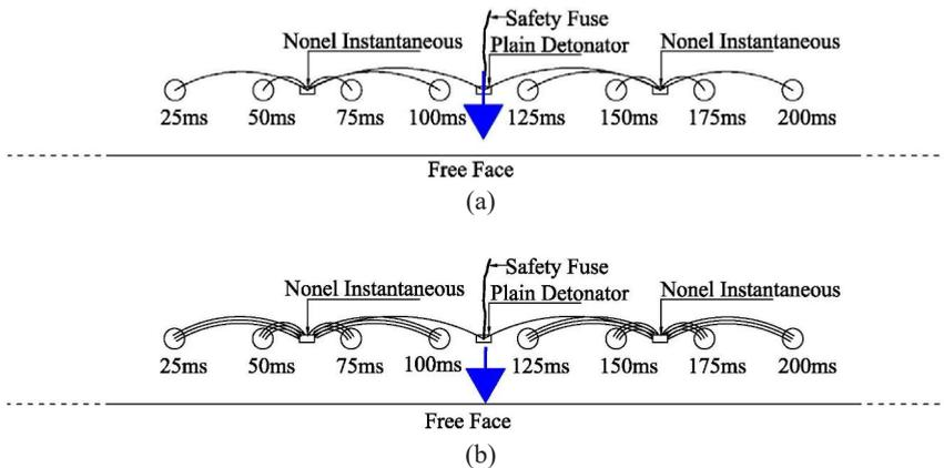
Fig. 7. Firing pattern for Bench-4: a) full-column charge b) multiple mid-air deck
