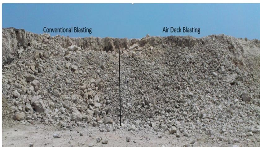
Fig. 14. Comparison of fragmentation of full-column charge blast and 20% multiple mid-air decks at Bench-4
