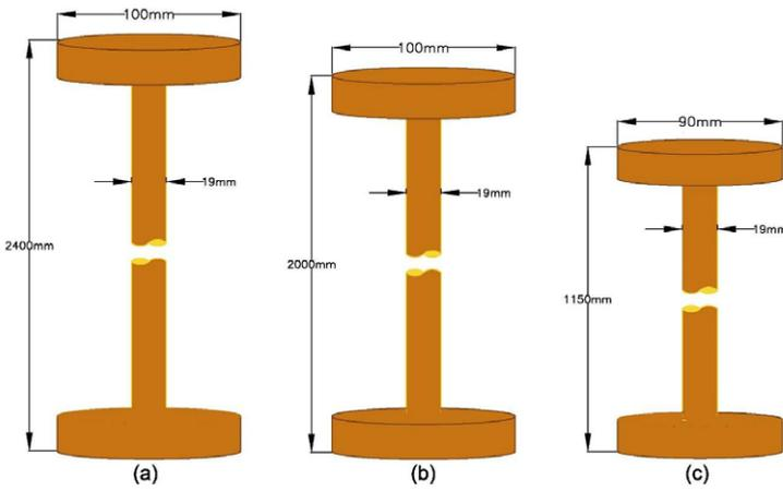
Fig. 2. Wooden plugs used as a spacer in (a) Bench-1 and Bench-2 (b) Bench-3 (c) Bench-4
