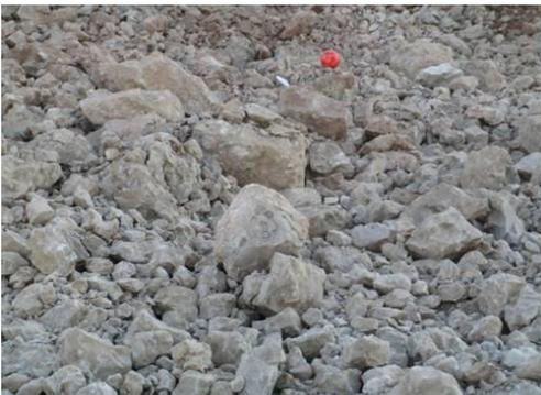
(c) Fragmentation of 20% top air deck blast at Bench-1
