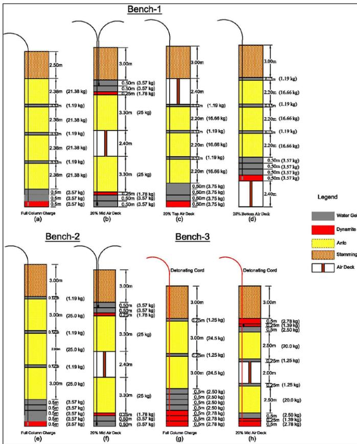
Fig. 3. Loading scheme of blast holes at Bench-1 (a-d), Bench-2 (e-f), and Bench-3 (g-h)
