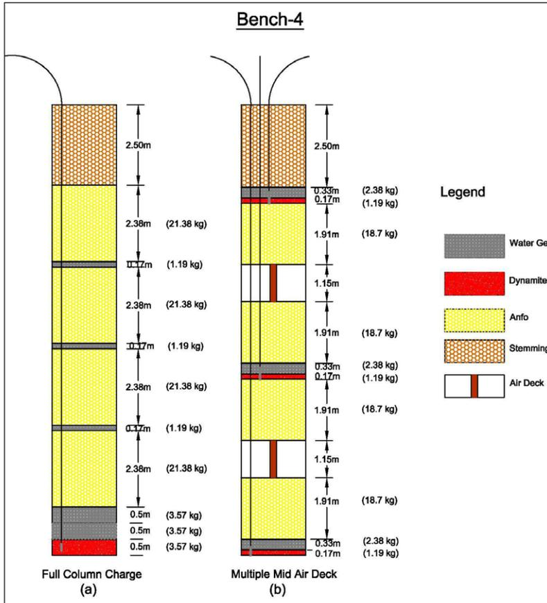
Fig. 6. Loading Scheme of blast holes at Bench-4 with (a) full-column charge and (b) with multiple mid-air deck positions
