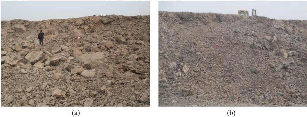
Fig. 12. Comparison of fragmentation of full-column charge blast and 20% mid-air decks at Bench-3
