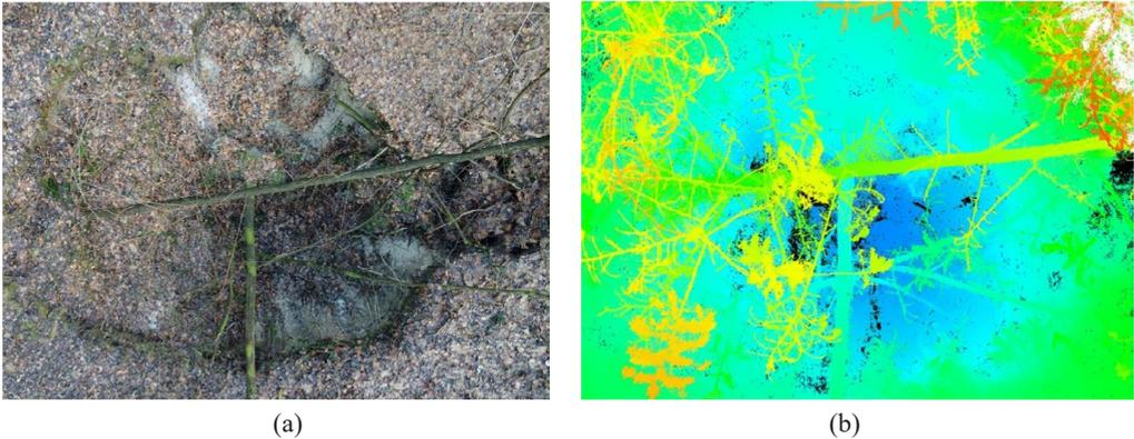
Fig. 5. a) TLS point cloud before filtration in RGB colours, b) TLS point cloud seen in reflectance intensity colours
