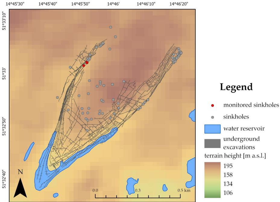
Fig. 3. Location of identified and monitored sinkholes in the underground mining study area
