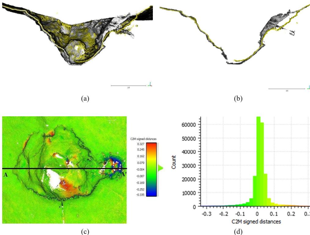
Fig. 7. (a) Visualization of a cross-section through the T1 TLS point cloud, (b) T5 data superimposed on T1 data, (c) DEM of difference (T1-T5), (d) histogram of distance differences between the point clouds T1-T5
