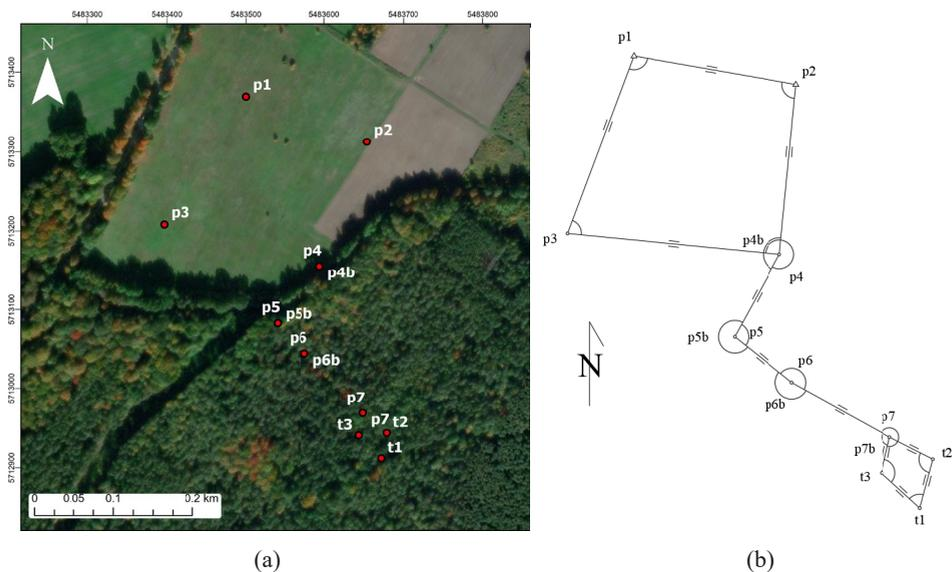
Fig. 2. Location of surveying grid points on the background of orthophotomosaic (a), sketch of polygon sequence (b)
