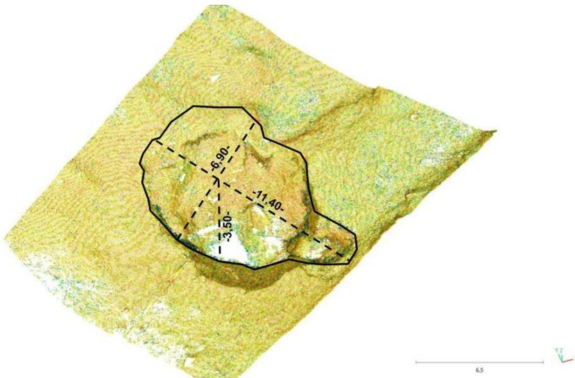
Fig. 6. 3D (isometric) view of the point cloud model of the sinkhole
