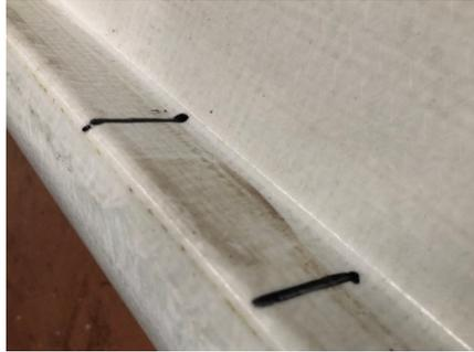
Fig. 15. A view of the rail and a mark left by the wheel – no indentations or material discontinuities
