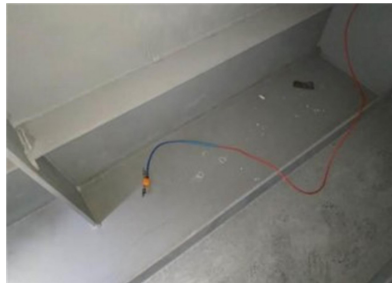
Fig. 7. Surface strain gauge placement diagram on the main beam
