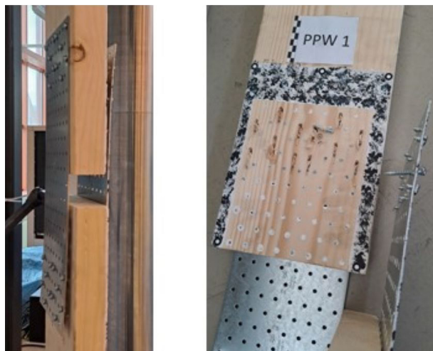
Fig. 11. Connection failure mode in group GB2
