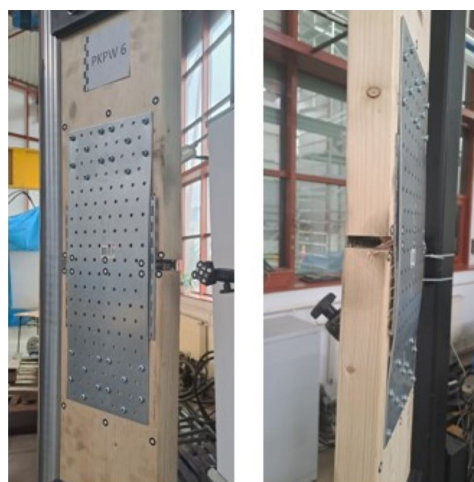
Fig. 12. Failure mode in Group GB3
