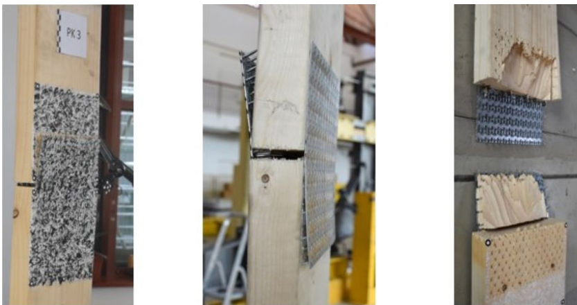
Fig. 10. Failure mode in group GB1: (a) pulling out of the spikes of metal plate fasteners, (b) symmetric form of failure, (c) block tearing
