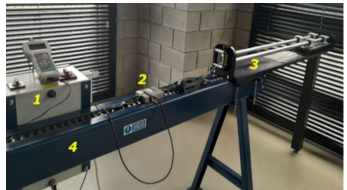
Fig. 2. Model cross-wedge rolling machine: 1 – data acquisition device, 2 – AXIS force measurement sensor, 3 – physical modelling module, 4 – chain drawing machine
