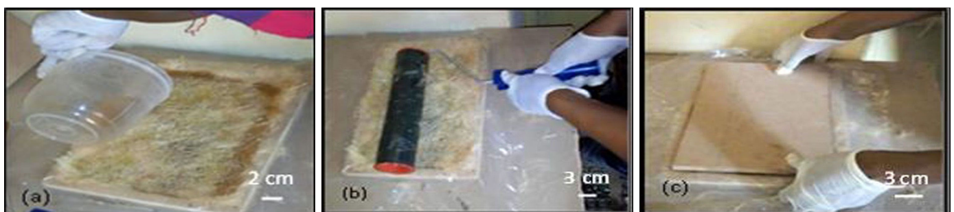
Fig. 6. (a) Impregnation, (b) Hand roller process, (c) Hand Layup finishing process
