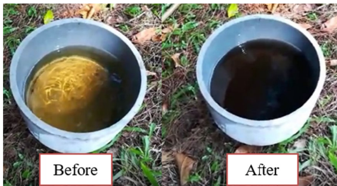
Fig. 3. The reaction of iron and sulfur turned the yellowish groundwater into black in 14 seconds
