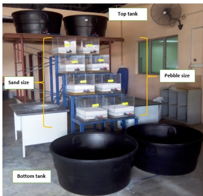
Fig. 2. Two rows of marble filtration system consist of pebble and sand-sized particles
