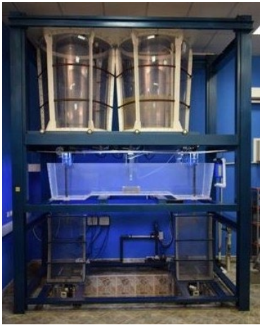
Fig. 2. 0.33 scale water model of two-strand slab tundish
