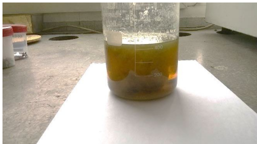
Fig. 5. Reaction mixture after the chemical removal of varnish layers from the tested steel sheet samples
