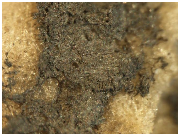
Fig. 8. Microscopic photograph of the deposited tin sponge. Image magnified 100 times
