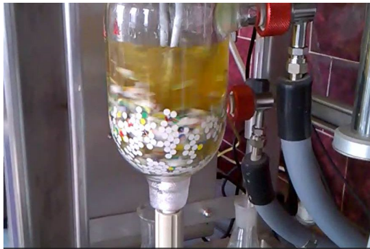
Fig. 3. Chemical removal of varnish and paint layers in a reactor. State after 1 minute of the process
