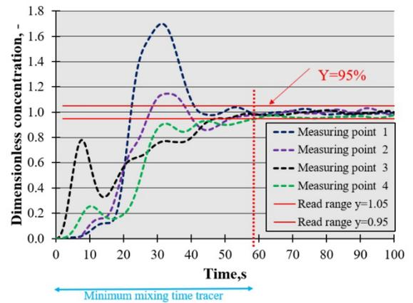
Fig. 7. Water model of mixing-time characteristics – variant B\_50\_37
