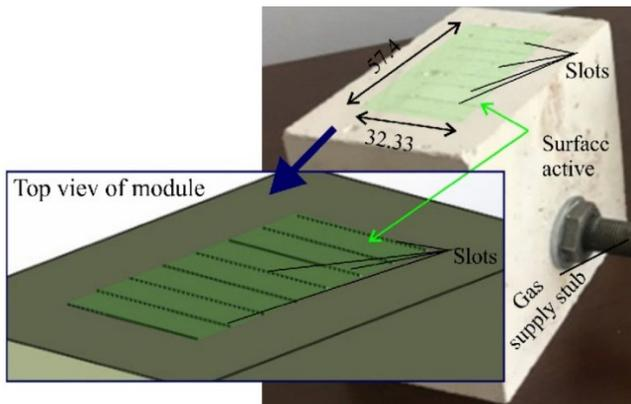
Fig. 3. View of the slot-type module (KS diffusor)
