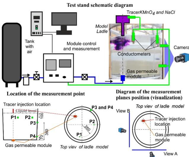
Fig. 2. Test stand schematic diagram (water model ladle)
