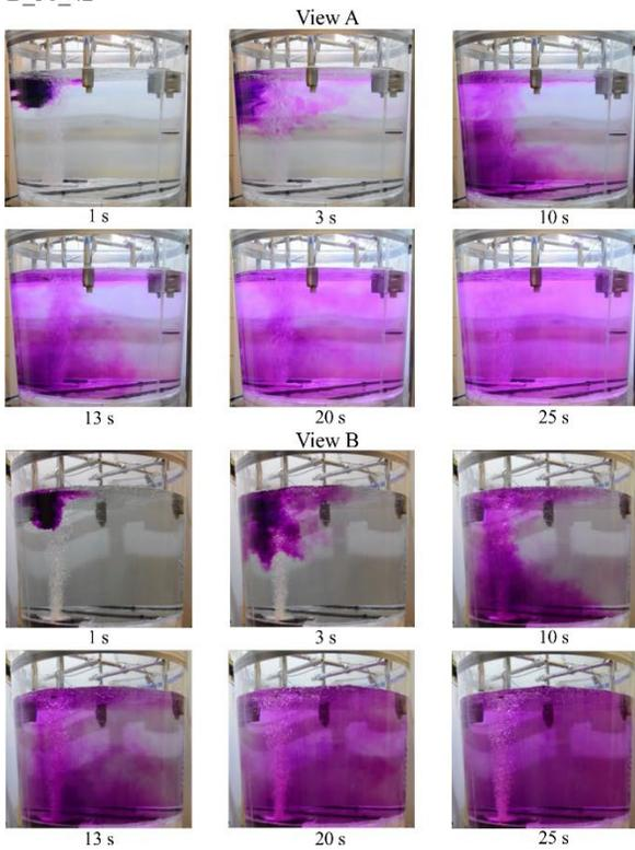
Fig. 6. Visualization of mixing in KS diffuser – type B depending on the experiment variant
