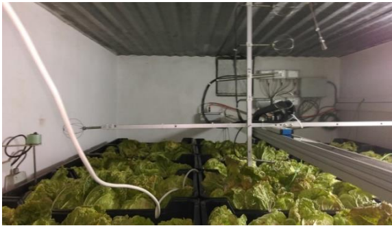
Fig. 1. Photo of the experimental cold store: view from the air cooler side. The elements of the mobile measurement system are visible.
