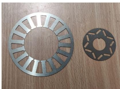
**Fig. 3.** Laminated stator and rotor developed motor
