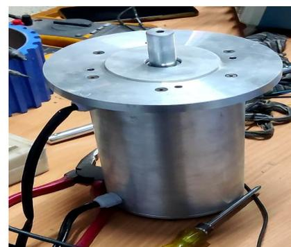
**Fig. 5.** Actual 48 V, 1.5 kW BLDC motor developed
