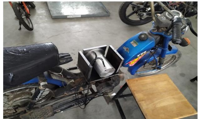
Fig. 19. Motor fitted in the frame
