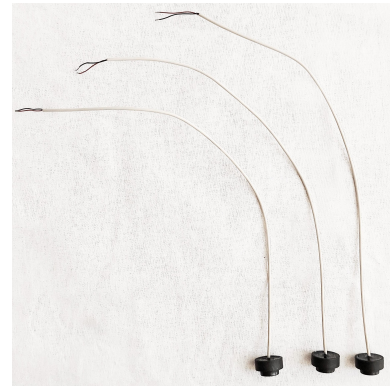
Fig. 5. Schematic of ultrasonic sensors with a central frequency of 1 MHz and a focal length of 66.74 mm.
