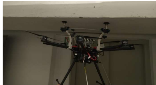
Fig.14. Drone after docking to the surveyed surface
