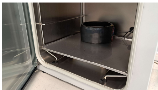
Fig.6. View of the designed solenoid placed inside of the incubator
