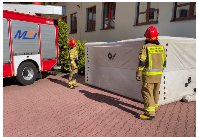
Fig. 1. Rescue cushion operated by Polish fire-fighters (source: National Headquarters of the State Fire Service of Poland)
