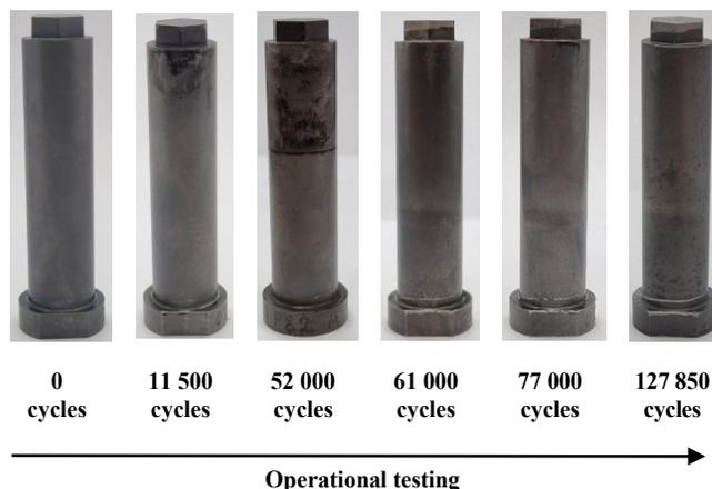
Fig. 5. Example of component A during operational testing
