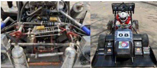
Fig.14. Decoupling suspension racing
