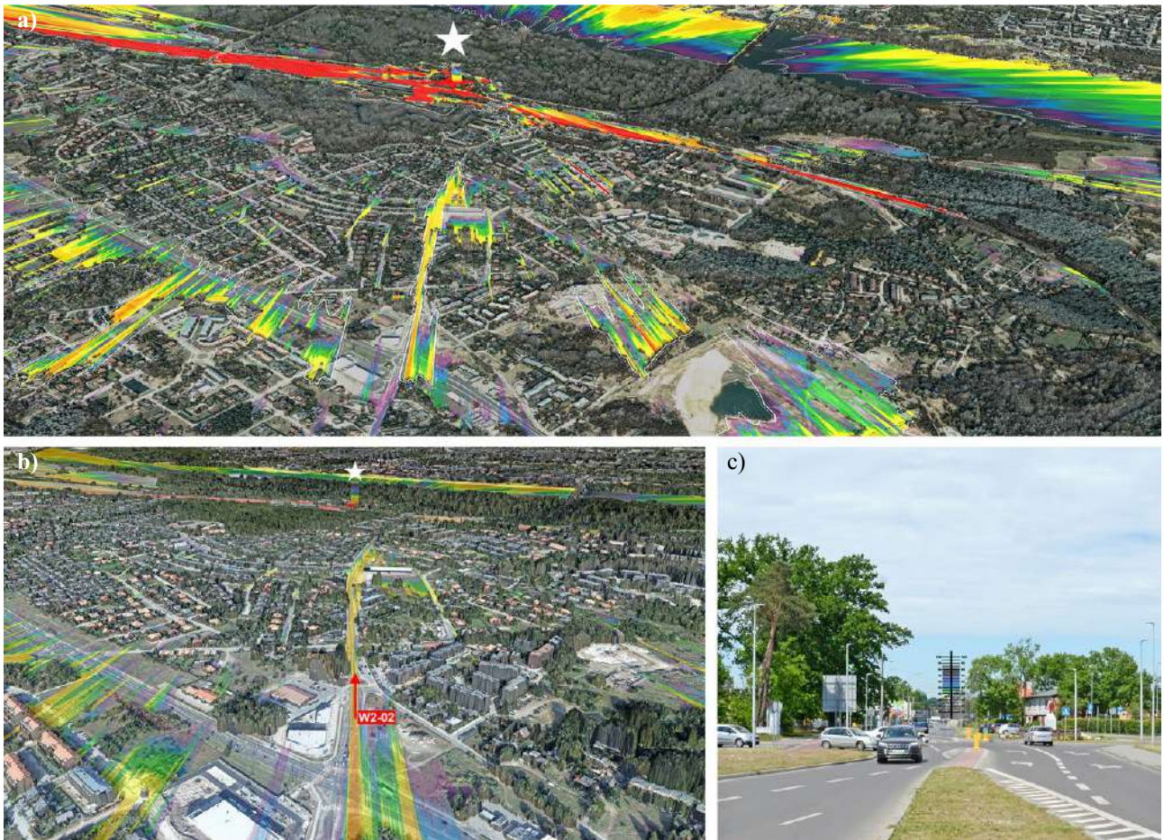
III. 7. Visual impact of the planned building in the southern part of the city: a), b) 3D model of the city with VIS analysis, c) simulation of the view from Łódzka Street using a height ruler.
