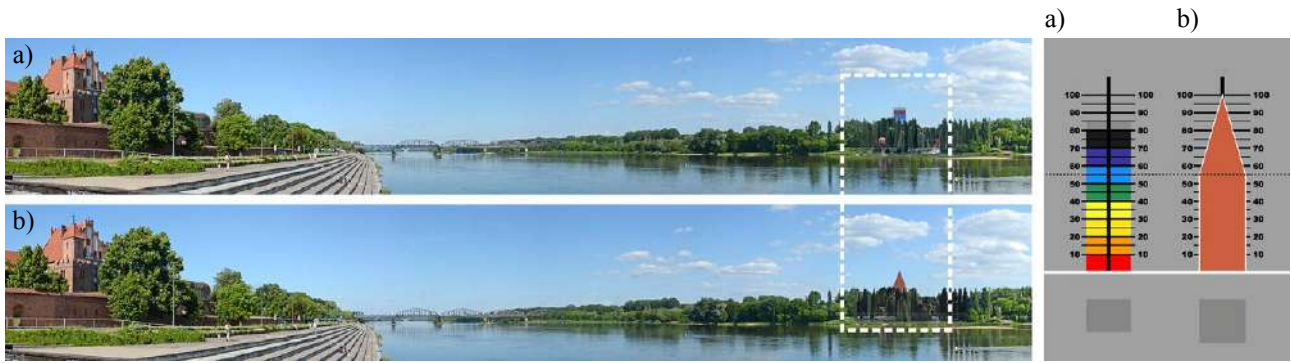
Ill. 5. Panorama showing the planned tall building in the wider cityscape. Different forms of the planned building were used in the simulations: a) rectangular form of 85 m, b) form that becomes slimmer with its height (block height of 100 m).
