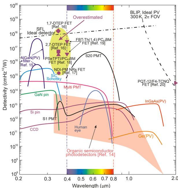
Fig. 1. Comparison of room temperature  $D^*$  for OSC photodetectors [14, 16–20] with standard market detectors (AlGaIn, Si, Ge, InGaAs PDs, and PMTs) in the wavelength range of 0.2–2  $\mu\text{m}$ . The ultimate SFL and BLIP are also shown. PV – photovoltaic detector, PMT – photomultiplier tube, FET – field-effect transistor. The OSC photodetectors  $D^*$  marked in magenta are overestimated.
