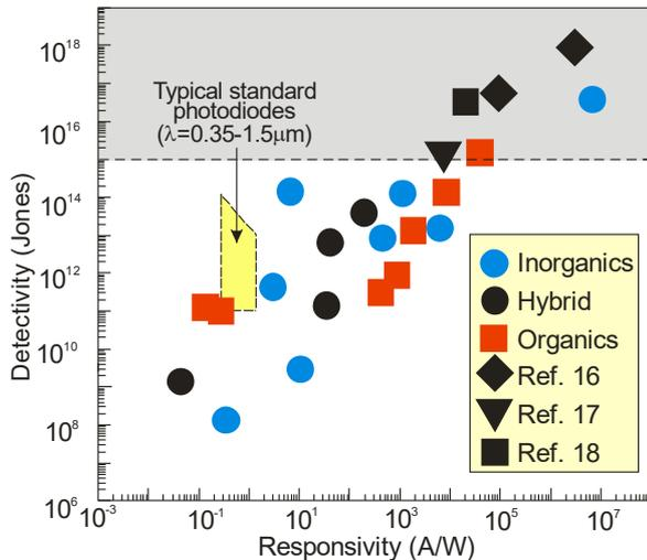
**Fig. 3.** Detectivity vs. current responsivity for visible-blind UV photodetectors presented in [17] and taken from [16] and [18]. The experimental data above the dashed line (in the grey box) are overestimated.
