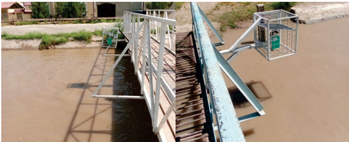
Photo 4. Smart devices for determining water flow installed on the irrigation canals (phot.: N. Ikramov)
