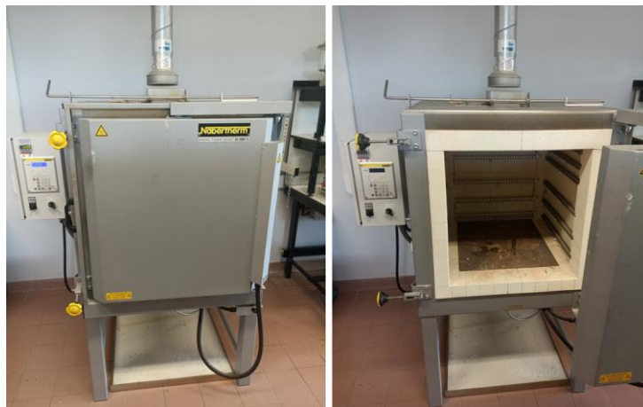
Fig. 6. Annealing furnace (Nabertherm LH 216/12)
