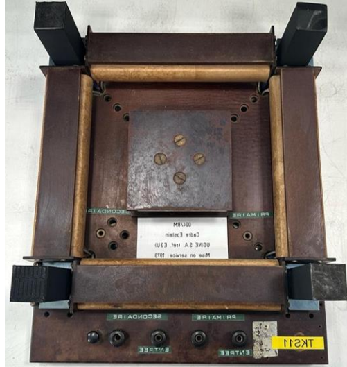
Fig. 3. Epstein frame for magnetic characterization
