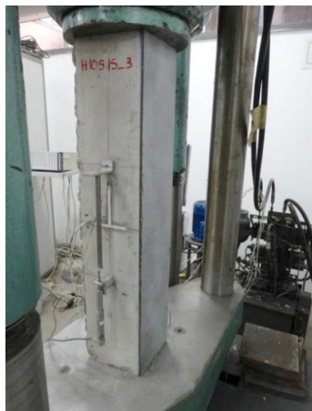
Fig. 2. Method of measuring concrete deformation and element shortening
