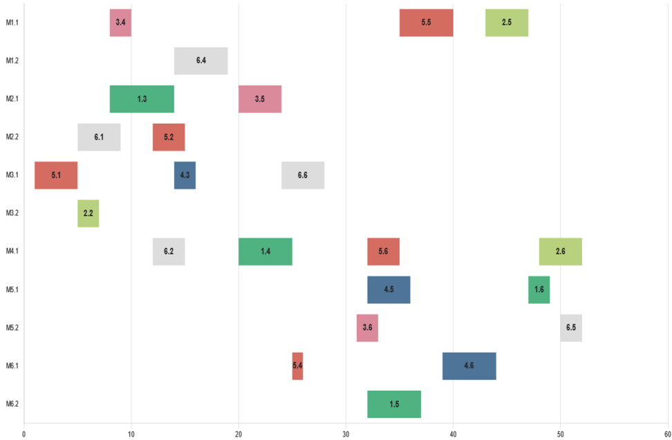
Figure 3: Gantt chart representing sequence-dependent setup times for the FT06 instance (FIFO) with machines operating at full efficiency ( ME(O_k^i) = 1 )
