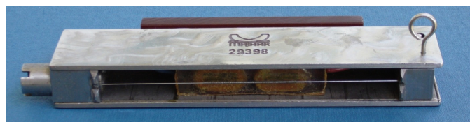
Fig. 1. Maihak strain gauge – measuring base 100 mm, range 0.2 mm
