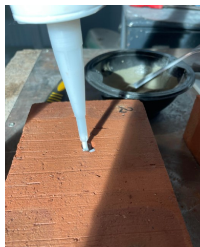
Fig. 4. Performing gravity injection in the brick with injection cream
