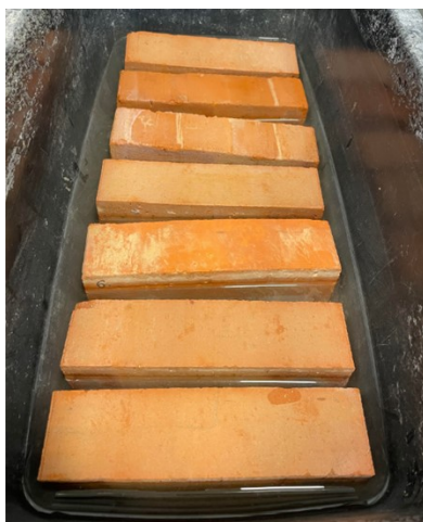
Fig. 3. A building caster containing bricks flooded with water to achieve adequate moisture content
