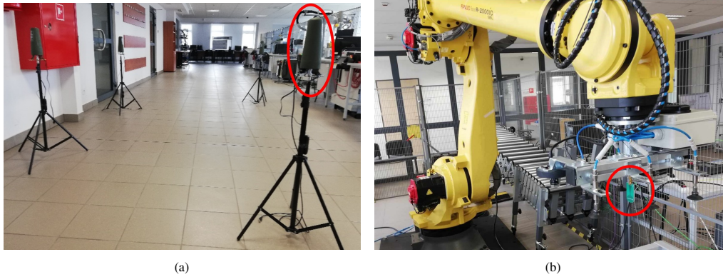
Fig. 4. The UWB beacons and the antenna module in the gripper of an industrial robot during experiments.
