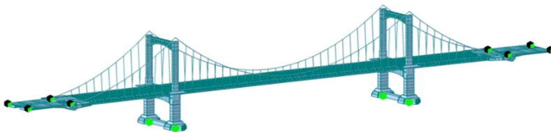
Fig. 4. Finite element model of self-anchored suspension bridge
