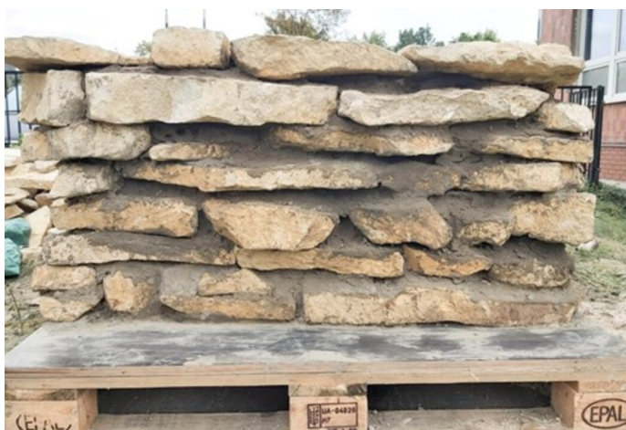
Fig. 10. Stone wall on mortar 3366-25C
