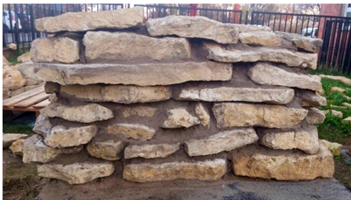
Fig. 9. Stone wall built with earth-based mortar without additives – composition 4060
