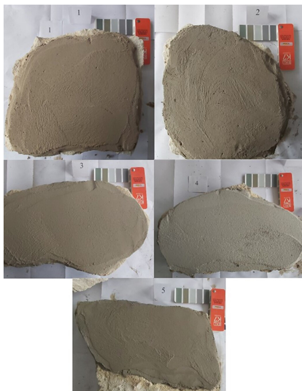
Fig. 6. Colour analysis of hardened mortars: 1 – 4060, 2 – composition 4060-15C-N, 3 – composition 3366-15C, 4 – composition 2575-15C-10L, 5 – composition 3366-25C
